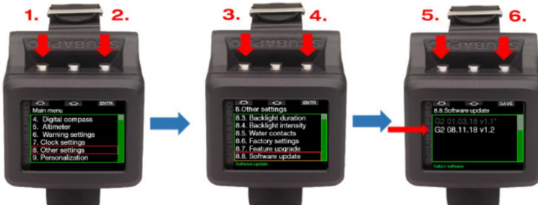
Repeat until you reach "8.8 Software update". Press the right button, choose the latest Software and save your changes by pressing the right button again. The Software currently installed on your G2 is marked by an asterisk [\*].
