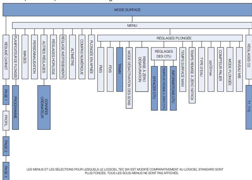
LES MENUS ET LES SÉLECTIONS POUR LESQUELS LE LOGICIEL TEC SW EST MODIFIÉ COMPARATIVEMENT AU LOGICIEL STANDARD SONT PLUS FONCÉS. TOUS LES SOUS-MENUS NE SONT PAS AFFICHÉS.
