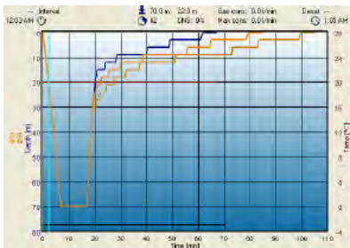
Figure 1 - Effect of MB level settings to the dive profile. MB 0 = blue, MB3=yellow, MB5=brown.
