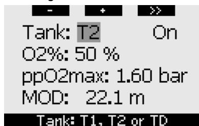
While **TANK** is highlighted, use the - and + buttons to choose the tank for which you want to set the oxygen concentration.
